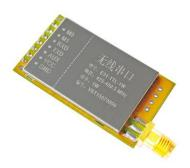
E31-TTL-1W is a 1W wireless transceiver module with narrow-band transmission, operates at 425-450.5MHz (default: 433MHz), based on original imported RFIC AX5043 from Switzerland, transparent transmission is available, WOR (ultra-low power consumption), TTL level. The outstanding advantages of narrow-band transmission is more concentrated power densities, longer transmission distance, and better anti-interference performance.
